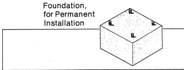
Mount the generator on a foundation if it is to be used as a permanent or standby power source. When planning a foundation, consider the following points:
