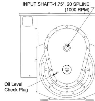
3. Remove the oil drain plug, drain the oil into a clean oil resistant container, 1 quart or larger. Check the oil for metal. Fine metal dust in the oil does not indicate trouble, but metal chips do. Dismantle the gearcase and look for damaged gears if you find metal chips in the oil.
