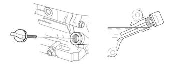
Oil is added to the engine by removing the oil cap and adding oil at this point. After filling the crankcase to the proper level, be sure you properly tighten the oil fill cap. NOTE: This engine generator must be on a level surface before you check or add oil to the system.
