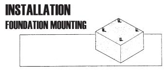
Mount the generator on a foundation if it is to be used as a permanent or standby power source. When planning a foundation consider the following points:
