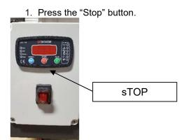
2. If not equipped with 2-Wire Start, move the on/off switch to the "OFF" position.
