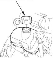
Oil is added to the engine by removing the oil fill cap and adding oil at this point. After filling the crankcase to the proper level, be sure you properly tighten the oil fill cap. NOTE: This engine generator must be on a level surface before you check or add oil to the system.
