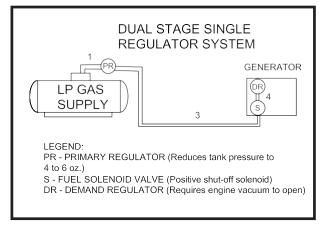
Reference numbers 1 through 3 in the block dia- grams above are system parts supplied by customer.
