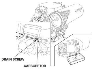
and yearly or 100 hours thereafter under normal operating conditions. Change engine oil every 50 hours of operation if the engine is operated under heavy load, or in high ambient temperatures.
