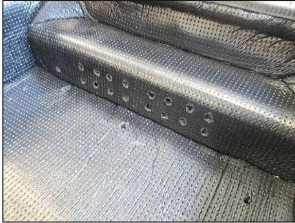
Sound-absorbing coating– Internal lower side
