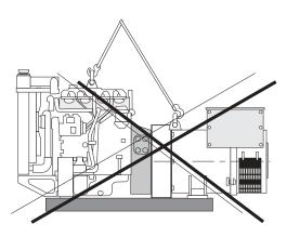
For single bearing alternator, the drive disc had been banded to flange with high intension strap wrench to avoid any touch between rotor and stator during the transportation. Please do not cut the strap wrench before you install the alternator with the engine.
