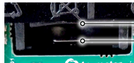
Install Battery Between These Two Points
