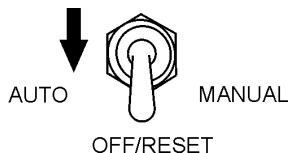
Figure 54. MPEC Control Switch (Off/Reset)
