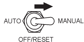
Figure 43. MPEC Control Switch (Manual Position)
