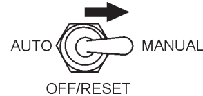
Figure 38. MPEC Control Switch (Manual Position)
