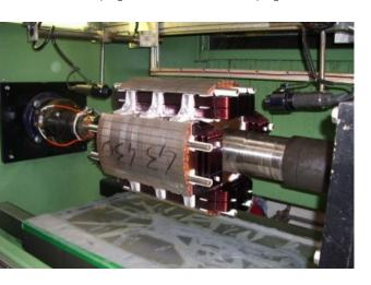
process is completed, a further protective varnish layer can be applied by dip or by spraying: the two varnishes that can be used are the grey EG43 or the black severe environment protection.
