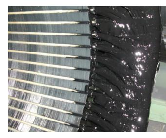
chemical attacks. Due to its encapsulation capability and durability, is also extremely resistant to the particle abrasion as it adsorbs the impacts. Moreover, this leads to a long-trouble less life protection, as the protection layer follows elastically the thermal expansion cycles of the windings from the cold to the hot condition and vice versa without forming any cracks.
