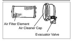
■ Cleaning the air filter element
