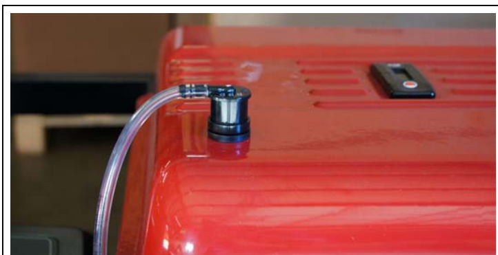
FUEL TANK “SLOSHING” VALVE INSTALLED
