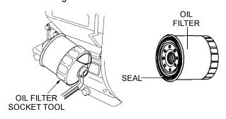
Figure 31. Oil Filter Removal
