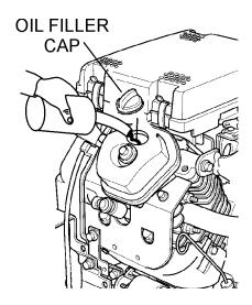
Figure 8. Engine Oil Filler Port
