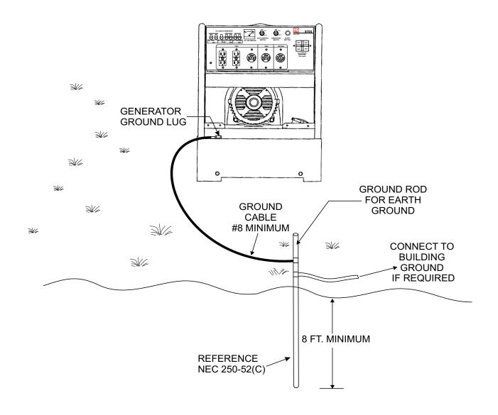
Figure 2. Generator Grounding
