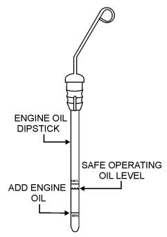
Figure 7. Engine Oil Dipstick
