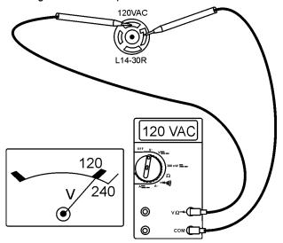
Figure 23. 120/240V Receptacle (120V)
