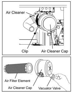
Cleaning the air filter element If dry dust is adhering : Blow compressed air from inside the element. If carbon or oil is adhering : Replace with new parts.
