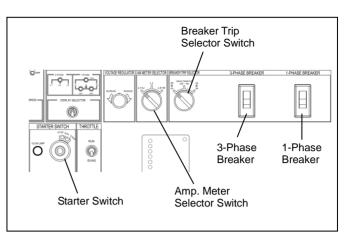
• Do not leave the generator in this RUN position with the engine stopped. Doing so will cause the battery to drain.
