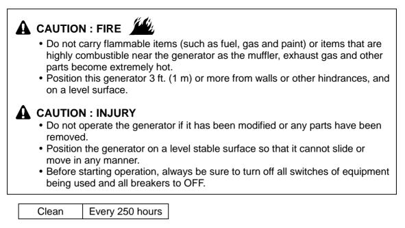
Accumulation of carbon (soot, unburned fuel) in the exhaust pipe line and muffler could cause only a system derates or an engine fault occurs. To destroy the soot and unburned fuel, run the unit at rated power for some period of time until the exhaust gas become mostly colorless every 250 hours operation time. The carbon will be easier to be generated when the unit operates at less then 30% of rated power. In this case, perform the above procedures at shorter interval time.
