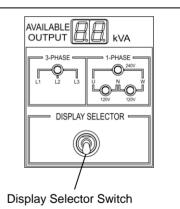
If "--" is displayed for the available output, it means that usage has exceeded the rated capacity. Immediately stop the equipment being used and reduce the load capacity of the equipment.
