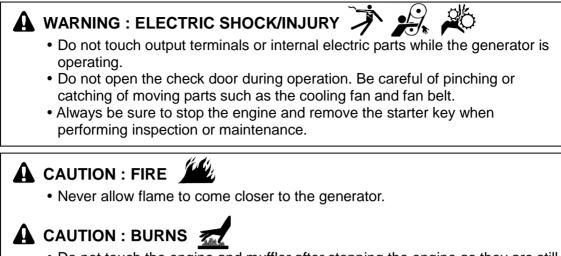
• Do not touch the engine and muffler after stopping the engine as they are still extremely hot.
