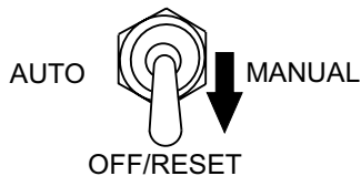
Figure 53. Auto-Off/Reset Manual Switch (Off/Reset Position)
