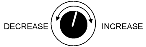
Figure 21. Voltage Regulator Knob
