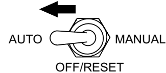
Figure 50. Auto Off/Reset Manual Switch (AUTO)
