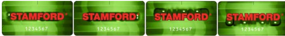
FIGURE 3. DOTS VISIBLE IN LEFT, RIGHT, UPPER AND LOWER VIEWS OF 3D HOLOGRAM
