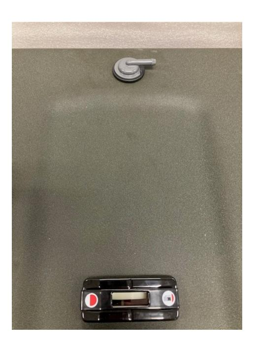
5. Add the fuel shutoff valve to the underside of the tank with fuel grade thread sealant. Note: do not over tighten.
