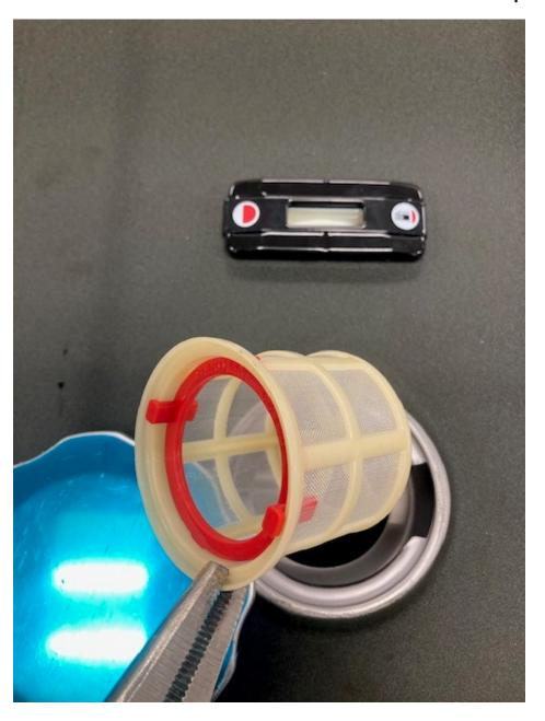
3. Replace chain with new cap chain. Replace strainer into tank. Note: new fuel cap has a pin hole in it for venting.
