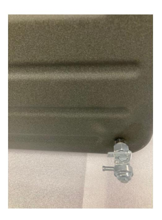
6. Use supplied fuel hose, clamps, and reducer to connect tank to your engine.
